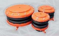
Air spring's support is provided by pressurized air within a thin walled rubber container similar to but lighter than the side walls of an automobile tire. As the sound is not transmitted by the air or the tire cord reinforced neoprene body, air springs could effectively eliminates the high frequency noise transmission.
